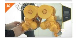
Pull off the peel ejectors.
