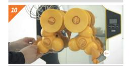
Pull off the peel ejectors.
