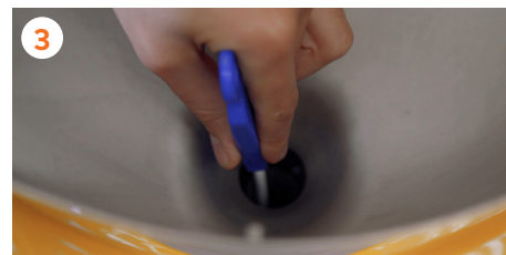
3 Insert the cleaning brush into the Drain&Clean hole in the base of the feeder, removing any residue that you may find in the tube.
