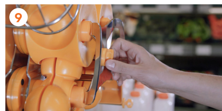
9 Unscrew the central knob of the Pressing Unit .
