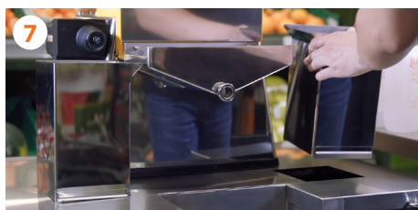
7 Remove the stainless-steel peel guides .
