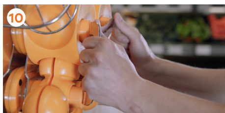
10 Remove the Pressing Kit by pulling it towards you with the stainless-steel handles.
