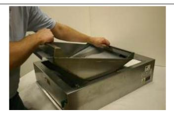
5. Use a nylon brush(a) to thoroughly clean grease and debris from holes in pan. Be sure to clean top and bottom of pan, pan divider, staging rack, and flat surface insert with hot soapy water. Rinse well and dry(b).
