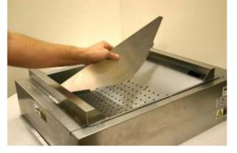
4. Remove the Pan by picking up on the front then lifting entire pan vertically.
