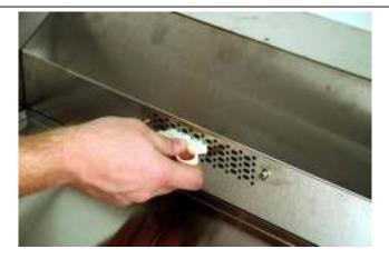
8. After brushing grid, use a clean cloth to wipe the debris and oil from grid and machine.
