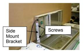
10. Hold the side mount bracket firmly against the Vertical Support Tubing and mark the holes in the center of each slot to be drilled with a 9/64" bit. Once drilled, insert and tighten screws provided (SCR008).
