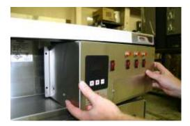
Depending on whether the Right Side well or the Left Side well is to be disabled, remove the power wires from the back of the power switch for that well. This would be wires #1 and #2 for the Left Side or wires #5 and #6 for the Right Side. Using the male connectors provided (F0243), cap these wires individually creating a dead end on each wire.
