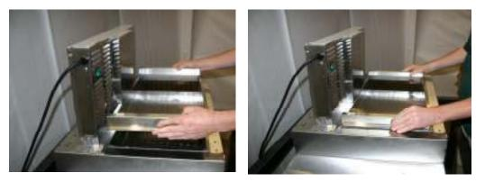
8. Plug electrical cord into power receptacle of the table.
