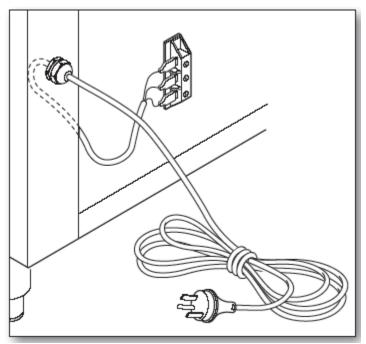
The flexible cable for connection to the electrical mains must not have characteristics which are less than those of a type with rubber insulation mod. H07RN F and it must have a section which corresponds with that set forth in the section "Technical Data" of the oven. The cable must also be anchored to the frame with the cable clamp, the screw of which can be reached through a hole in the frame. It must in any case
