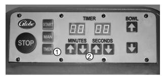
Press and continuously hold the up arrow buttons to the desired minutes and seconds. Press and continuously hold, the button scrolls through the number cycles guickly. (To slow down the selection and to better control the setting time, press the up or down arrow button do not continuously hold the button down).
