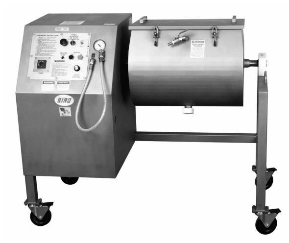
The BIRO VTS-100 VACUUM TUMBLERS are versatile machines used for vacuum tumbling all types of meats with marinaded blends of herbs and spices. All marinades should be FDA approved and meet F.S.I. standards. The BIRO VTS-100 produces equally impressive results with beef, pork, poultry and fish.
