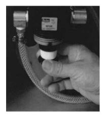
4. Separate the filter from the filter holders. Replace with a new filter.
