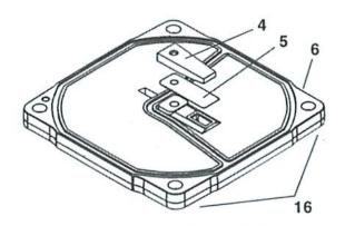
Valve Plate Assembly (available separately) (Valve Plate Assembly also includes items 7 & 8 as shown in the main exploded view)
