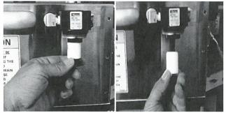
2. Unscrew the filter holder. Lower the filter carefully from the mounting stud. Note the order of the parts.
